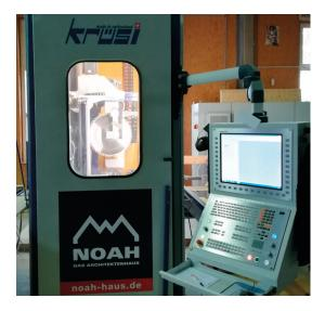
After import of the construction data, the individual parts are prepared for the CNC in a self-determined order, the CNC programs are generated fully automatically, and they are transferred to the machine.
