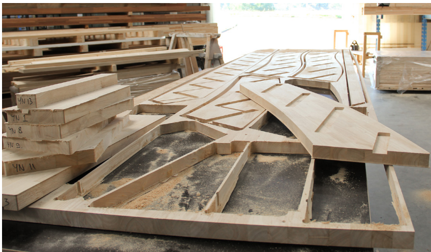
CPI saves about 20% of material by using the nesting method.
