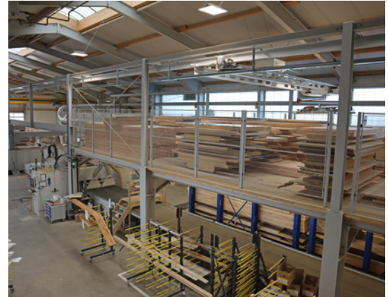
With a warehouse on the 2nd floor of the workshop, the existing space can be used twice.
